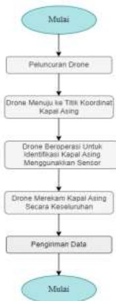
Gambar 4. *Flowchart* Cara kerja Drone ‘AeroEnforce’
