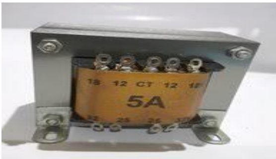
Figures5Travo/ Transformer (5 A cd 0-12 V)
